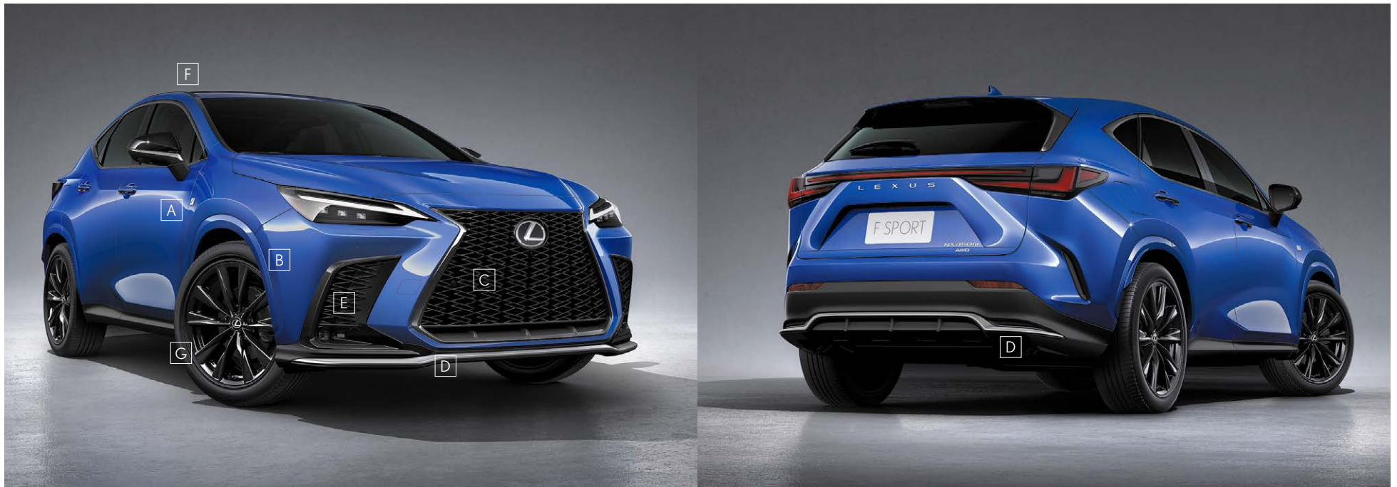
A_F SPORT emblem / B_Fender arch mouldings / C_Grille / D_Lower bumper spoiler / E_Garnish / F_Roof rails (black) / G_Exclusive 20" aluminium wheels
